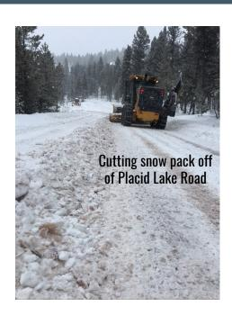
When ice forms on roads and the temperatures stay below freezing preventing ice melt, graders often show up to 'chip' away at the ice packs.
